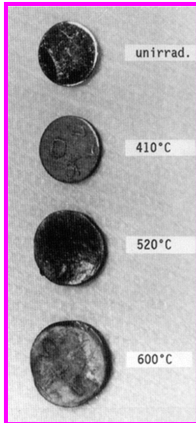
Neutron-induced swelling of V-alloys (H. Matsui, et al.)
