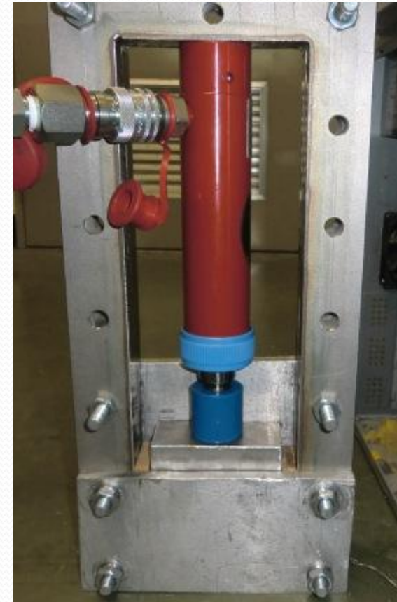
The pebbles were applied pressure by a hydraulic jack (30kN)
