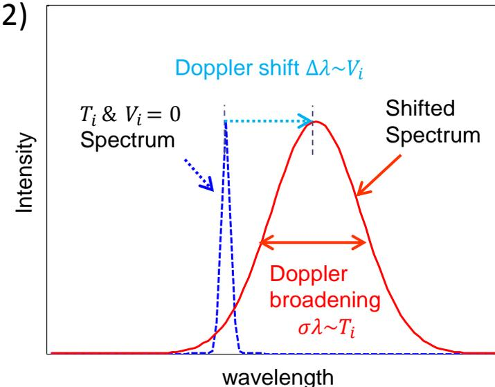
Fig.2. Schematic view of Doppler shift and Doppler broadening
