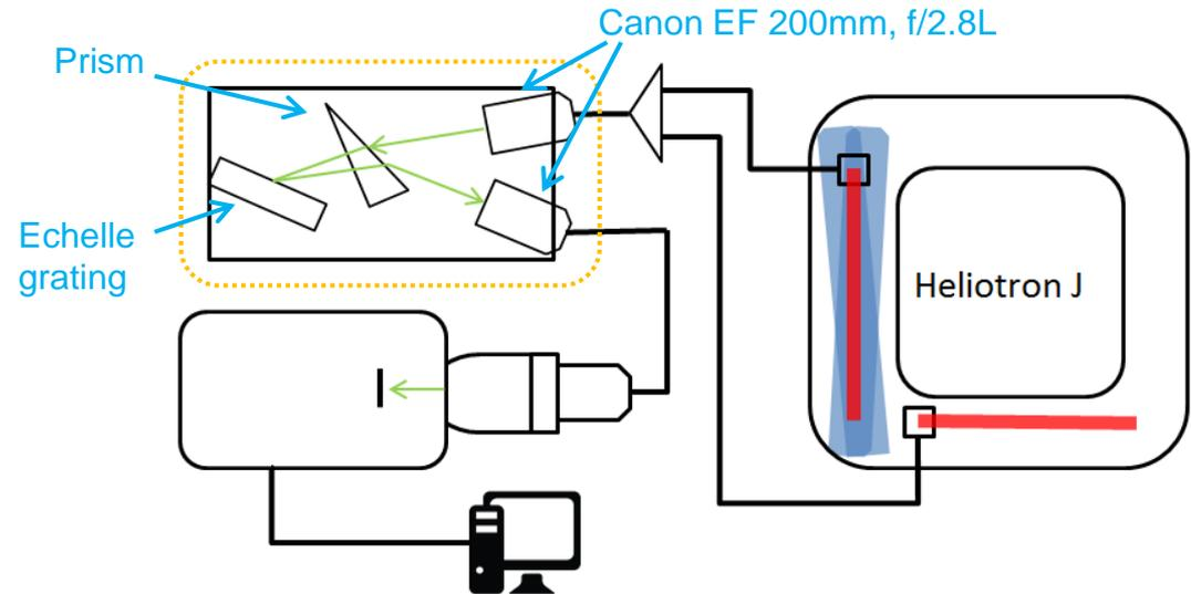
Fig.6. The Echelle-grating monochromator
