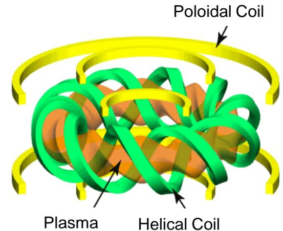
Fig. Schematic view of Tokamak device (a) and Stellarator device (b, c)
