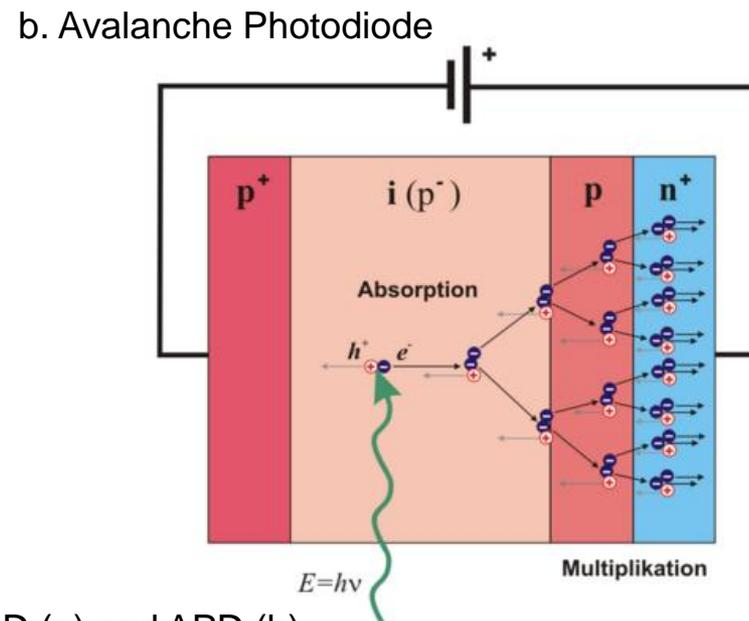
Fig.3. Schematic view of CCD (a) and APD (b)
