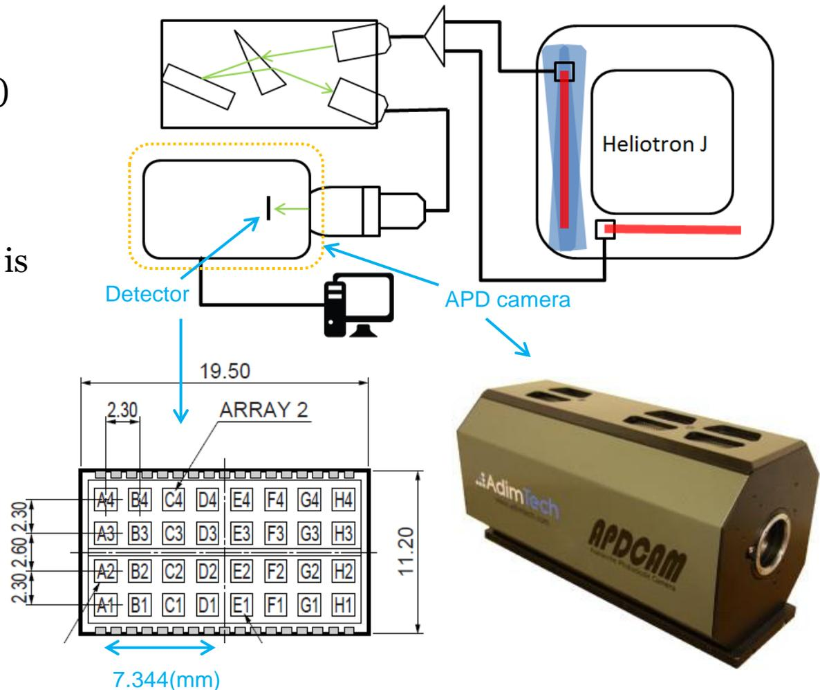
Fig.8. The APD camera and  $4 \times 8$  element APD array
