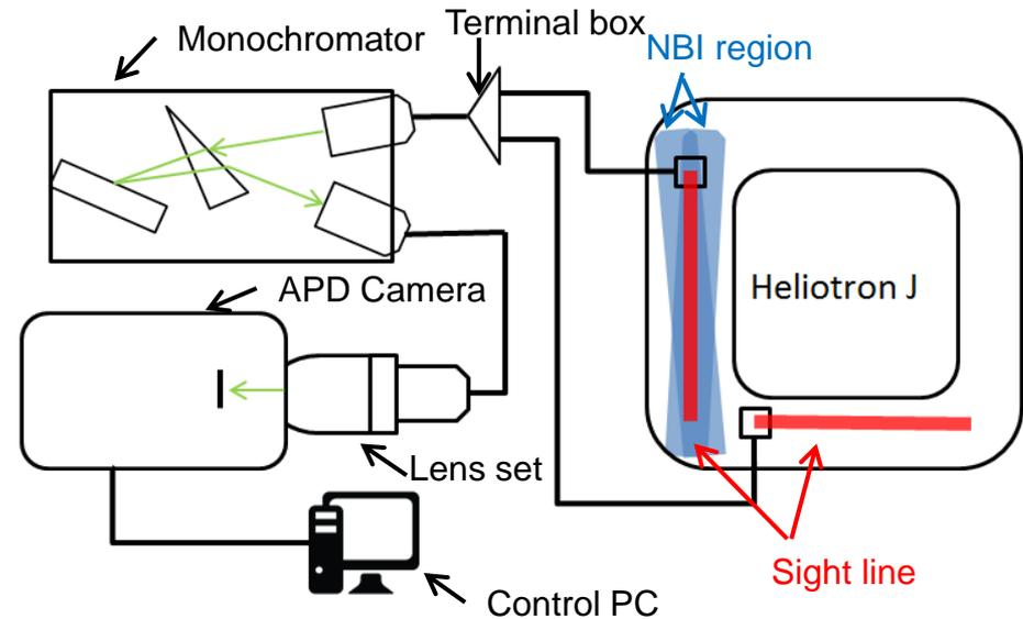
Fig.4. Schematic view of Ultrafast CXRS System
