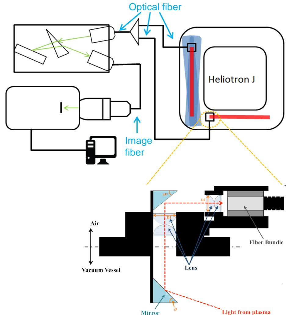
Fig.5. Schematic view of observation port
