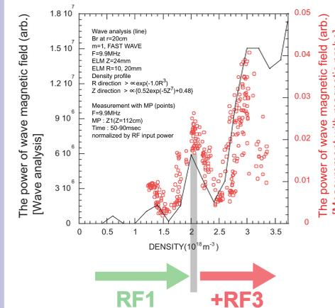
The power of excited waves was measured with the magnetic probe for the frequency 9.9MHz(RF1). The power of excited waves was also estimated from the calculation at the several radial locations. In the figure, measured values (red points) are plotted with the calculation (solid lines).
