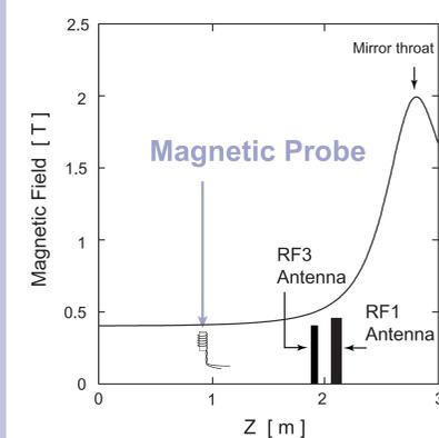
The power of the waves excited by RF1(9.9MHz) was measured using the magnetic probes located in the central cell.
