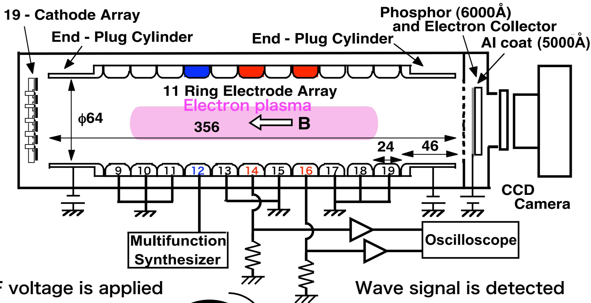
RF voltage is applied to 4 sector-electrode at **No.12**.
