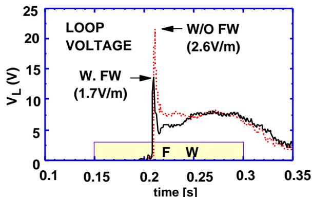
Fig.II.1-5 Time evolution of loop voltage with and without fast wave start-up assist.
