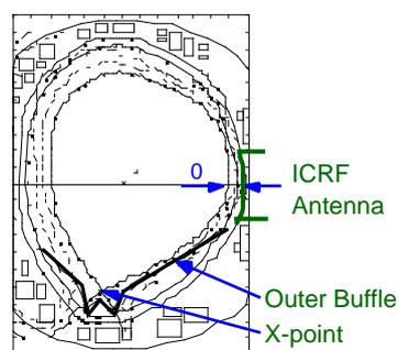
Fig. I.1.5-2 Configuration with W-shaped divertor for ICRF coupling
