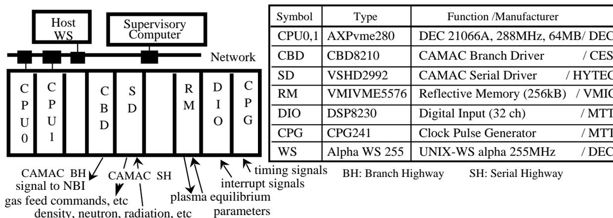
Fig. I.1.2-2 Configuration of the plasma realtime control system.
