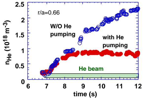
Fig. 1.2.6-1 Time evolution of measured He density with and without He pumping. The He density with He pumping reaches a saturation level at 1.2 s after the start of the He beam injection.
