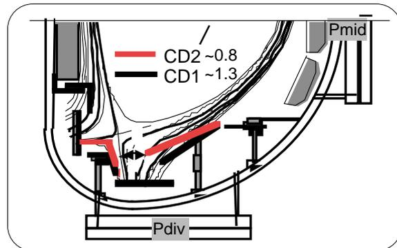
Fig. II.1-1 Variation of divertor closure on JFT-2M
