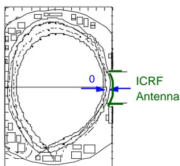
Fig. I.1.5-1 Configuration with open divertor for ICRF coupling
