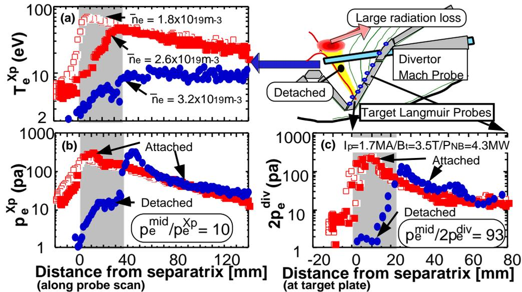
Fig. I.2.5-1 Plasma temperature and pressure profiles for attached and detached divertors.
