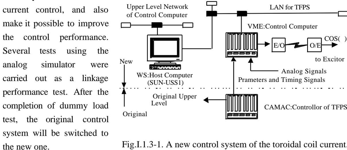
Fig.I.1.3-1. A new control system of the toroidal coil current.
