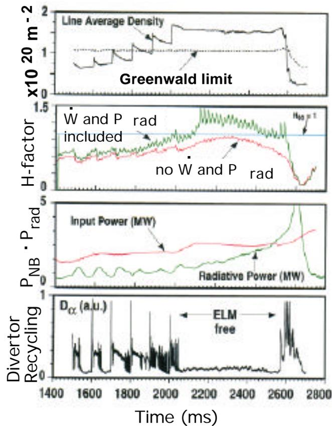
Fig. IV.3.1-1 Discharge waveforms of RI-mode
