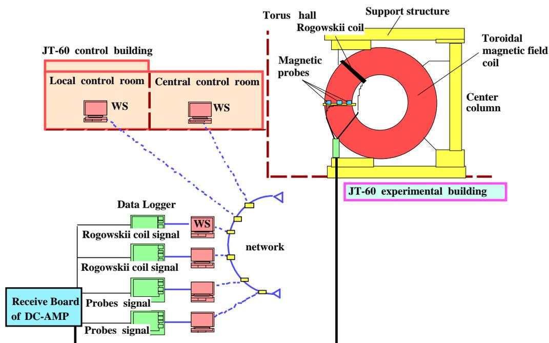
Fig. I.1.1-1 Short circuit detection system
