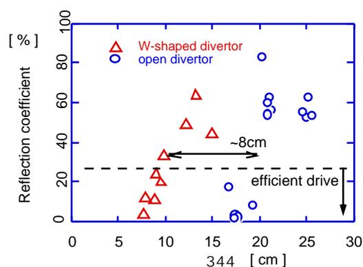
Fig. I.1.5-4 The reflection versus distance 344.
