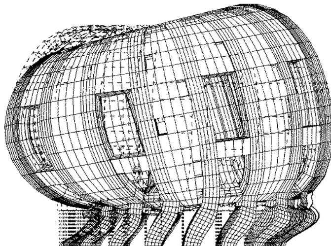
Fig.I.3.2-1 Model of superconducting coils for vibration analysis in JT-60SU;  $n=1$  vibration with 16.2Hz
