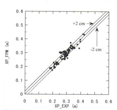
Fig. I.1.2-3 Correlation of X-point positions,  $X_{P-FPM}$  and  $X_{P-EXP}$ . ( $X_{P-FPM}$ : the FP formula on experimental data.  $X_{P-EXP}$ : the equilibrium analysis).
