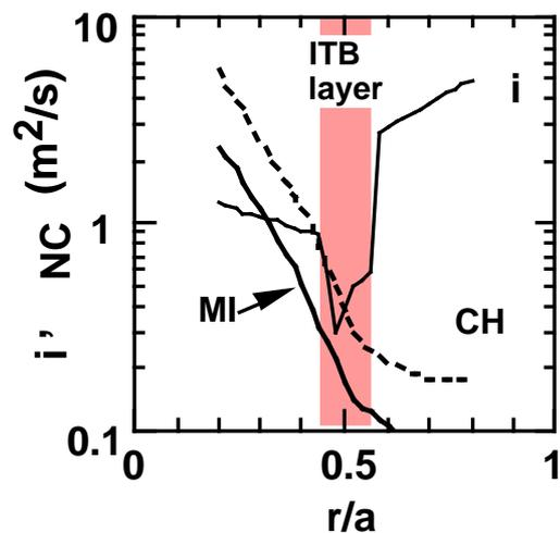
Fig.III.1-1 Profiles of ion thermal diffusivity,  $i$ , and neoclassical diffusivity,  $NC$ , evaluated by MI method and by Chang-Hinton's formula in the reversed shear plasma with internal transport barrier (ref. [1-1]).
