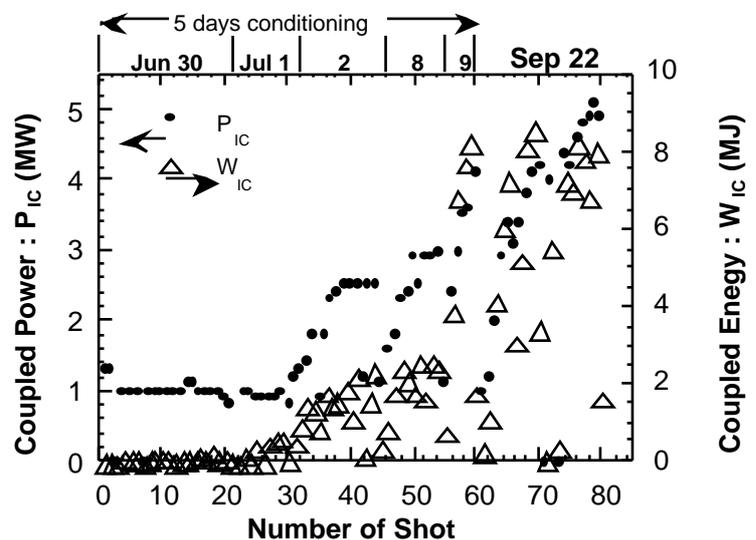
Fig. I.1.5-3 Progress of the coupled ICRF power and energy with W-shaped divertor.
