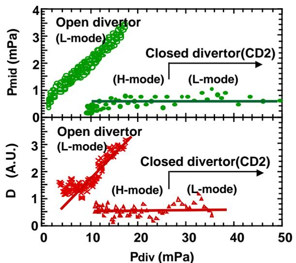
Fig. II.1-2 Correlation between midplane pressure,  $P_{mid}$ , and divertor pressure,  $P_{div}$ , with open and closed divertor (The recycling light from outer edge of the main plasma,  $D$ , also shows similar trend as  $P_{mid}$ )
