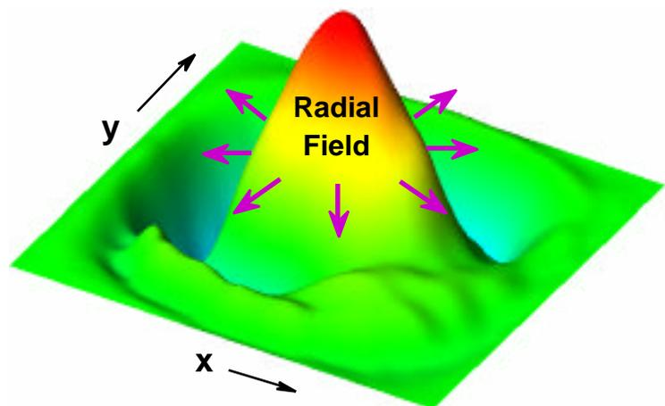
Fig.III.4.2-1 The electrostatic potential profile on a toroidal cross-section.  $m/n=0/0$  mode (radial electric field) induced by the nonlinear interaction grows to the same level as the 1/1 mode.
