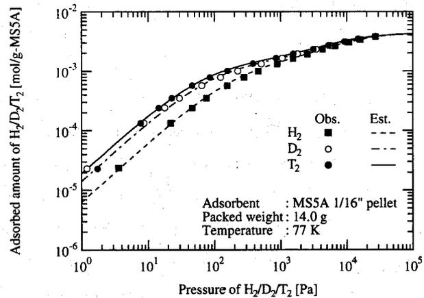
Fig. VII.4.3-1 The adsorption isotherms of H<sub>2</sub>, D<sub>2</sub> and T<sub>2</sub> on MS5A at 77 K.
