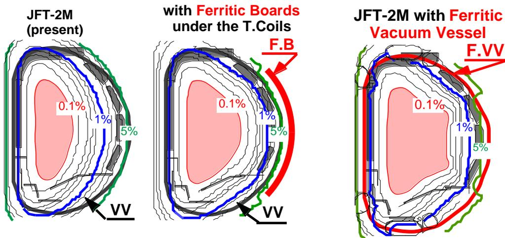
Fig.II.1-6 Equi-ripple-amplitude region in the cases of the nonmagnetic VV without (present VV) and with ferritic board.
