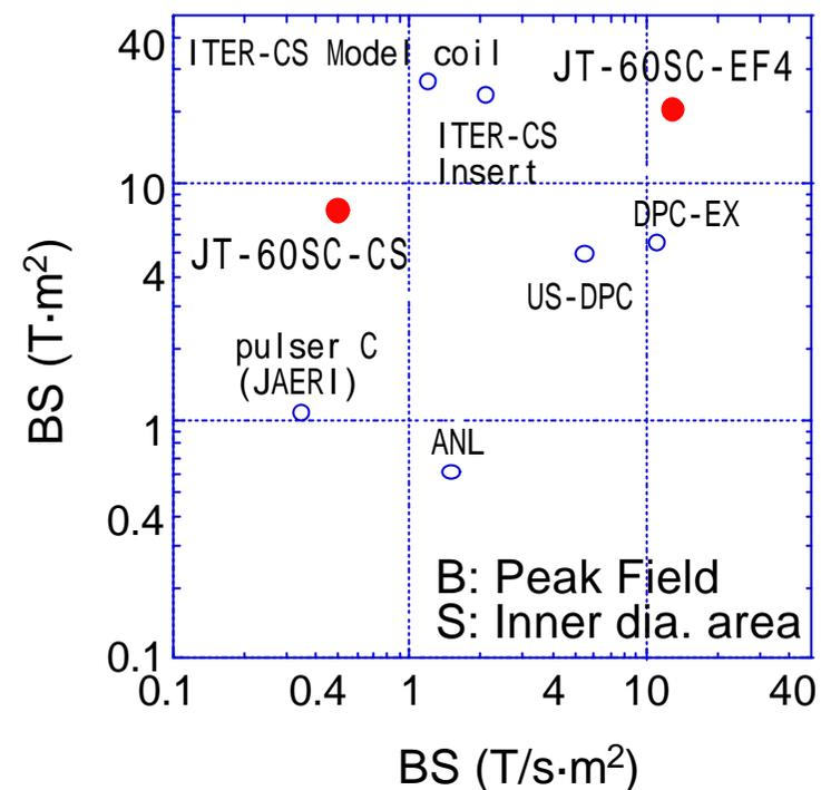
The PF coil system of JT-60SC will be one of the largest flux swing coils among coils in the world.
