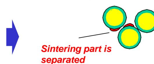
Interstrands resistance will be increased by mechanical cyclic load due to electro-magnetic force.
