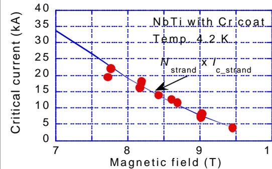
Measurement result of critical current of the full-size sample shows good agreement with value expected from the strands.
