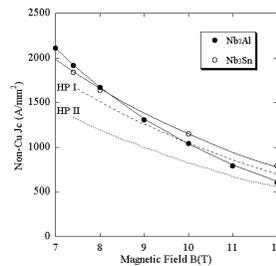
The non-Cu Jc for the developed Nb<sub>3</sub>Al (closed circle) and Nb<sub>3</sub>Sn (open circle) strands at 4.2 K.
