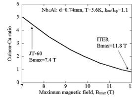
Maximum magnetic field dependence of Cu/non-Cu ratio.
