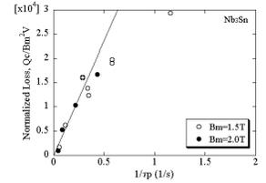
The inverse of ramping time ( $\tau_p$ ) dependence of normalized Qc of Nb<sub>3</sub>Al and Nb<sub>3</sub>Sn CIC conductors.
