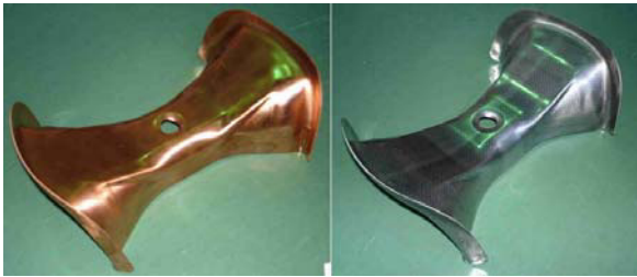
Figure 2: Press forming of half-spoke with 1.5 mm thick plates of copper (left) and aluminium (right).
