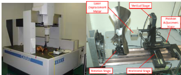
Figure 8: Precise 3D measurement device of ZEISS UPMC850 at KEK (left) and simple 3D measurement device made with the laser displacement sensor and optical stages (right).
