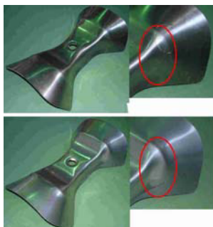
Figure 4: Deformation with the plates of 2.5 mm (top) and 1.5 mm thick (bottom).
