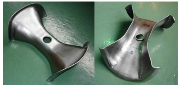
Figure 7: Press formed shape after burring with niobium sheet of 2.5 mm thick.
