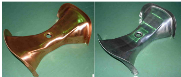
Figure 4: Press forming of half-spoke with 1.5 mm plates of copper (left) and aluminum (right).
