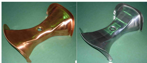
Figure 2: Press forming of half-spoke with 1.5 mm thick plates of copper (left) and aluminum (right).
