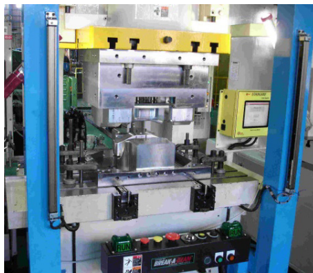
Figure 1: Assembled die set was mounted to press machine.
