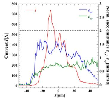
Figure 4: Current and horizontal and vertical normalized slice emittances in the bunch at the exit of the 1<sup>st</sup> arc. The broken line indicates the projected horizontal normalized emittance.
