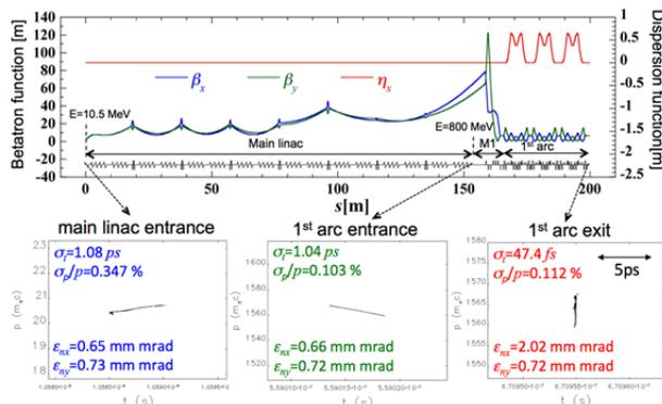
Figure 3: Betatron and dispersion functions from the main-linac entrance to the 1<sup>st</sup> arc exit (upper) and the time-momentum distributions with the basic beam parameters at the main-linac entrance, the 1<sup>st</sup> arc entrance and exit (lower).
