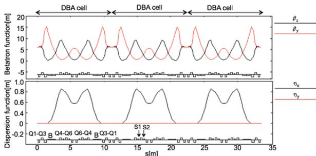
Figure 2: Betatron and dispersion functions of the 1<sup>st</sup> arc with three DBA cells having  $\beta_{x2}=1.0$  m and  $\alpha_{x2}=1.6$ .
