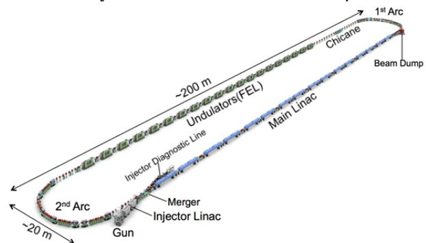
Figure 1: Image of the designed ERL-based EUV-FEL.
