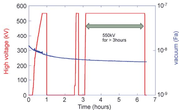
Figure 4: HV test without central stalk with additional ceramics at the cERL. Red is high voltage and blue is gun vacuum.
