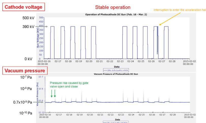
Figure 1: Typical gun cathode voltage and vacuum pressure during two weeks of the cERL operation.
