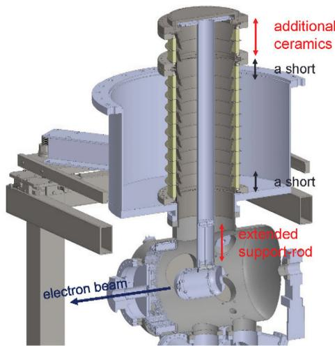
Figure 3: Gun configuration with additional two segmented ceramics at the cERL.
