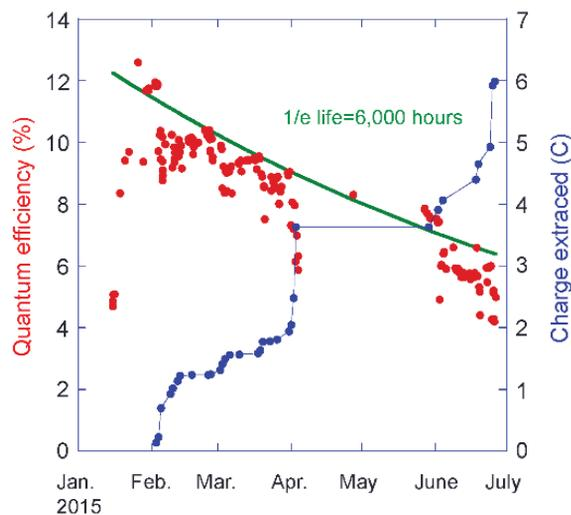
Figure 2: Quantum efficiency of GaAs photocathode and charge extracted during the cERL commissioning from January to July in 2015.
